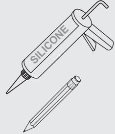
Cut out worktop to supplied dimensions shown in (fig 1) with suitable equipment and seal the cut edge as appropriate sealant.
